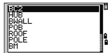
When the instrument is rebooted, the code stack is cleared.
