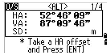
5. To calculate the coordinates and the raw data of the target point, press **[ENT]**.
