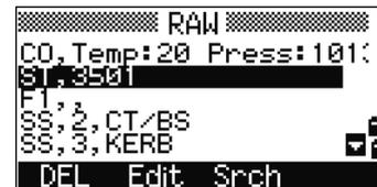
You can edit any field in the ST record, but the instrument does not recalculate any measurements from this station.
