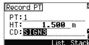
To assign a new feature code to a numeric key, press **[^]** or **[v]** to highlight the code that you want to change. Then press the **Edit** softkey.
