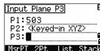
If the plane is defined by two points (by selecting **2Pt**), the vertical plane is the same as the plane used in the V-Pln function, but the indicating factors are **Sta** and **dZ**, not **a** and **b**. For more information, see [Measuring distance and offset values on the vertical plane, page 78](#).
