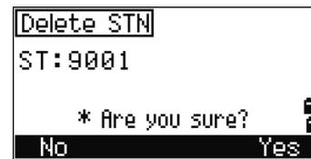
A reconfirmation screen appears. Press the **DEL** softkey to confirm deletion.
