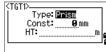
HT can be left blank in the target set. If you leave it blank, the current HT value is always applied to the measurement.
