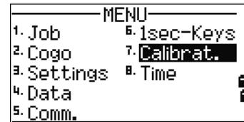
1. The Nivo series has two-axis level compensation. Take an F1 measurement to a target on the horizon. Press **[ENT]**.
