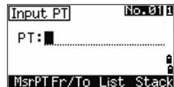
Enter the start point name in the Fr field and the end point name in the To field. You can include letters and hyphens in the point names, but the last character must be numeric.
