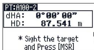
dHA            Difference in horizontal angle to the target point
