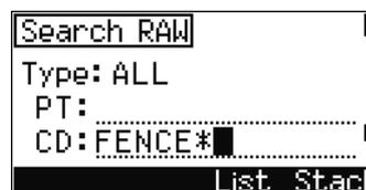
To search by point type, move to the Type field and use **←** or **→** to change the selected point type. The options are ALL, ST, SS, SO, CP, CO, CO(SY), and CO(RDM).
