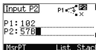
To continuously calculate a new point, enter +Ang, HD, and dVD from the previous bearing line. This is a convenient way to enter Traverse points.
