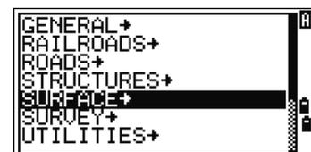
A layer has an arrow at the end of the code label. If you highlight a layer in the list and then press **ENT**, the codes and layers in that layer are displayed.
