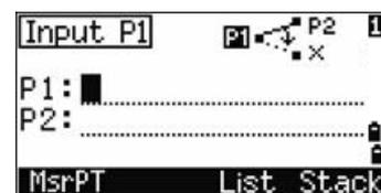
The input coordinates are used in the calculation. They are not saved in the database.
