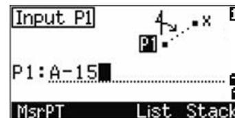
Enter the azimuth, horizontal distance, and vertical distance. Then press **[ENT]**.
