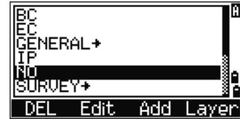
An editing screen appears. For points, the Edit Item screen appears. It contains only the PT field. For codes, the Edit Code screen appears, containing the CD field and the REC field.
