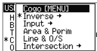
To assign a specific function from the sub-menu, press **[^]** or **[v]** to highlight the function. Then press **[ENT]**.
