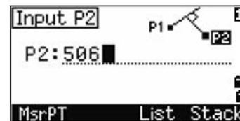
If P1 and P2 are 3D points, the Z coordinate of the perpendicular point is calculated relative to the P1-P2 slope.
