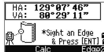
If you have taken a distance measurement to the center of the circle, press the **Calc** softkey to calculate the offset using one edge angle observation.
