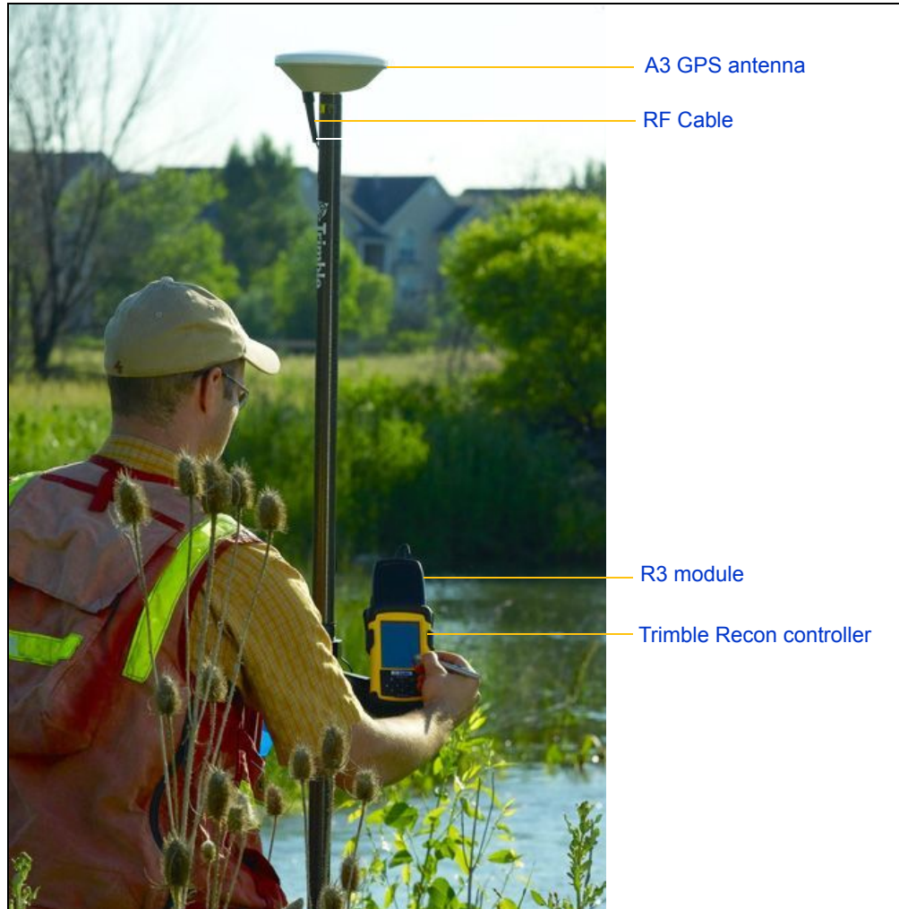
Figure 3.2 R3 system shown mounted on a survey pole.
