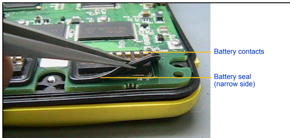
Figure 6.6 Seating the battery seals (gaskets)
