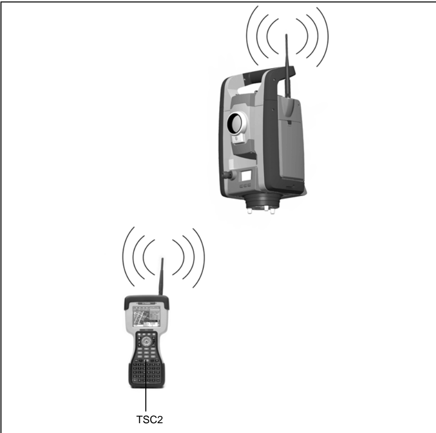
Figure 4.41 TSC2 connected to the VX Spatial Station using the integrated radio for robotic measurements.
