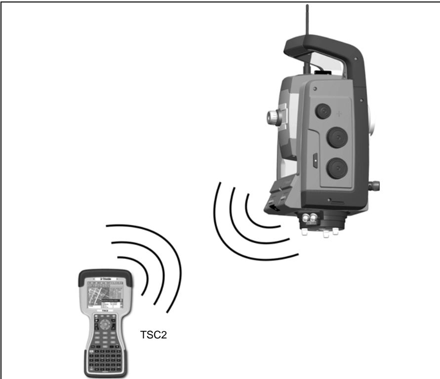
Figure 4.40 TSC2 connected to the Trimble VX Spatial Station with Bluetooth wireless technology for servo and Autolock measurements.
