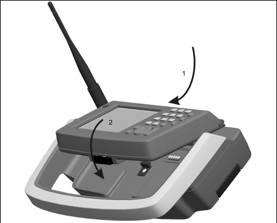
Figure 7.73 Attach Trimble CU to Trimble Robotic Holder
