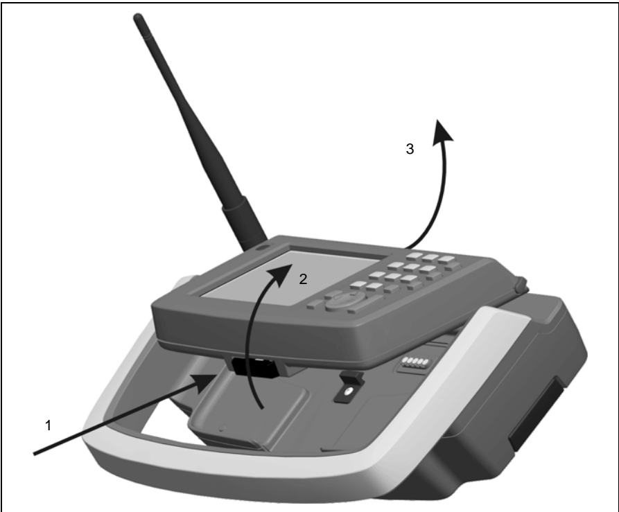
Figure 7.74 Detach Trimble CU from Trimble Robotic Holder
