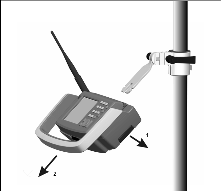
Figure 7.76 Detach Trimble Robotic Holder from standard rod adapter
