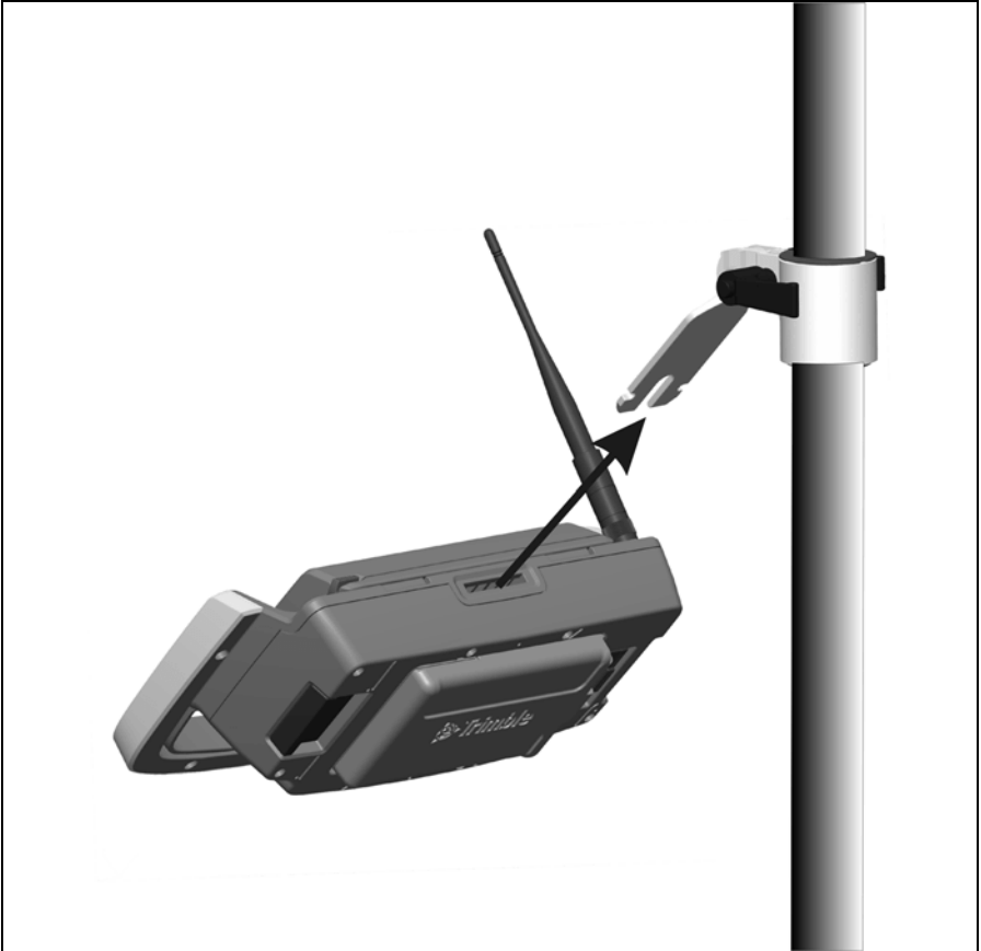
Figure 7.75 Attaching the Trimble Robotic Holder to the standard rod adapter
