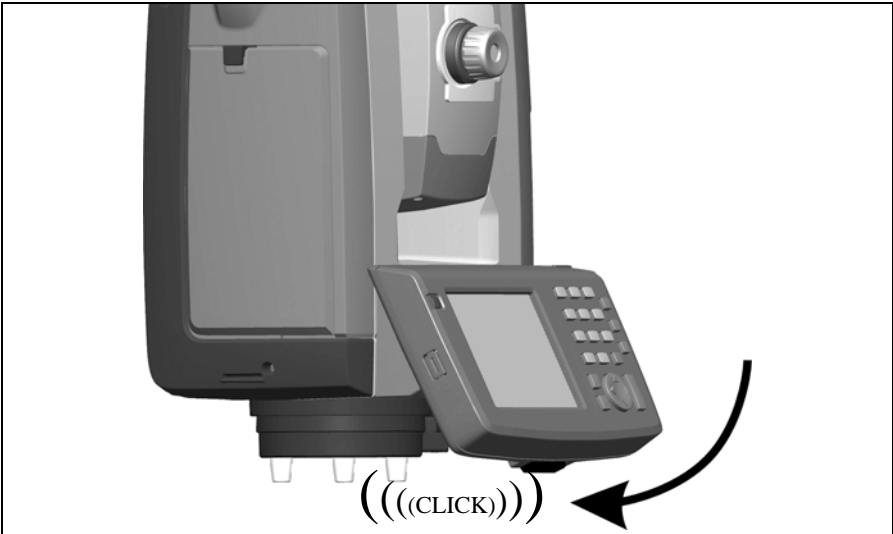
Figure 4.36 Attaching the Trimble CU
